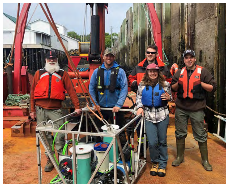
Photo: Researchers from Dalhousie University, Memorial University, and SOAR preparing for deployment of a multi-instrument bottom lander to monitor fish, Grand Passage, N.S., Photo Credit: SOAR
